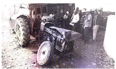
Prima facie cause of the accident: While a Tractor with trailer was plying in downhill gradient of the haul road in an opencast coal mine, the front left wheel of the tractor detached from its axle due to collision with a rock boulder of the berm, resulting into toppling of the tractor due to jackknifing, thereby inflicting serious bodily injuries to its operator and helper, which proved fatal to the operator and helper escaped unhurt.
