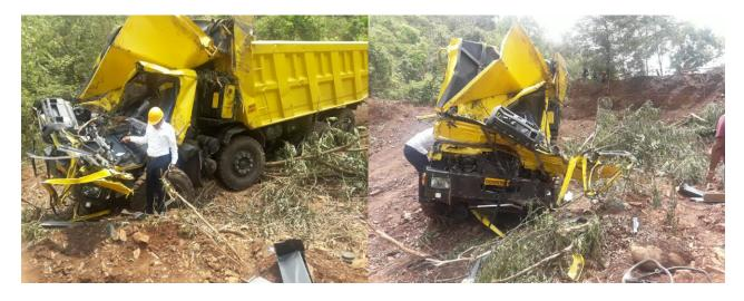
Prima facie cause of the accident: Loaded tipper transporting iron ore crossed the berm at the turning on the left side of the haul road and toppled down causing fatal injury to two persons.
