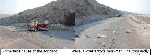
While a contractor's workman unauthorisedly drove a tractor inside an opencast workings, which is prohibited by order, it toppled hitting a boulder on the berm of a haulroad to which he received head injuries and succumbed after 64 hours at hospital.
