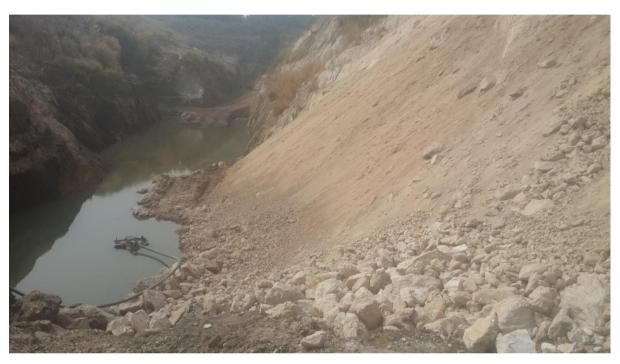
Prima facie cause of the accident: While a group of four persons were installing a pump at the bottom of an opencast manganese mine, located at a distance of about 3m from the toe of a slope of an overburden bench having height of about 12m, suddenly a loose boulder of approximate size of 1m x 1m x 0.5m rolled from the slope, broke into pieces and hit two of them, who received serious injuries to which they succumbed almost instantaneously and the other two escaped unhurt.
