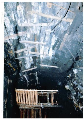
Prima facie cause of the accident: While a group of three persons were standing near side of a pillar in an underground coal mine, suddenly a piece of coal measuring about 1.50m(length)X0.20m(width)X0.40m(thick) fell from the side from a height of about 4.05m on
