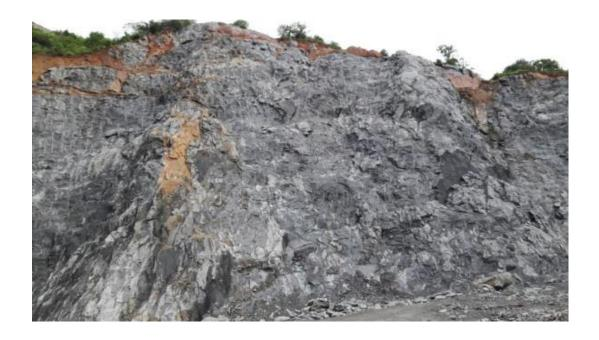
Prima facie cause of the accident: While a driller was drilling shot holes with jack hammer drill in an opencast stone mine, standing on a ledge of 0.7m wide and 3.5m high, without anchoring his safety belt, he had lost balance in the process and fell down through a height of 3.5m, sustaining serious bodily injuries, to which he
