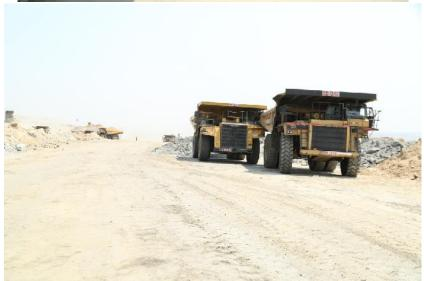
G Prima facie cause of the accident: "While an Operator was driving a loaded Dumper(100T) on the way to Dump yard, his Dumper hit another Dumper(100T) parked on a side of the same haul road, resulting damage to his dumper's cabin and serious injury to himself"
