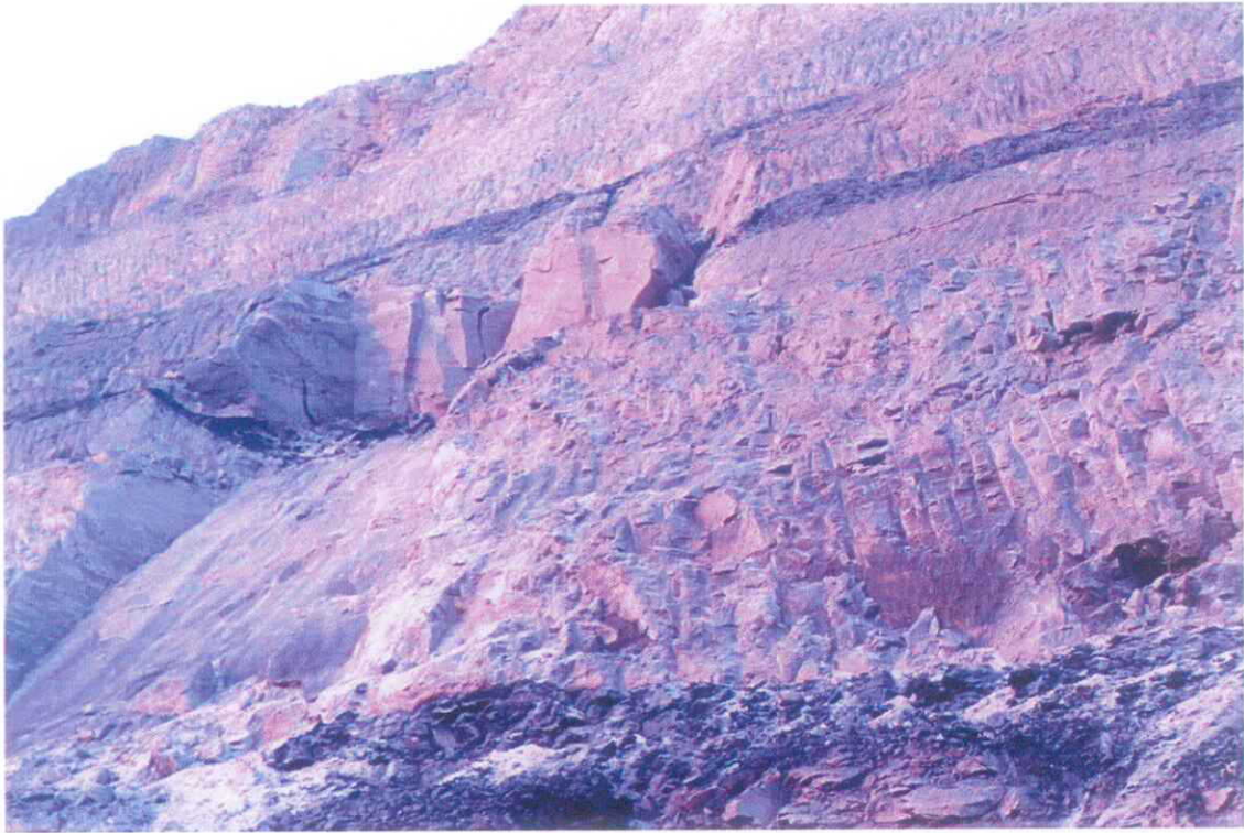
Photograph showing slide of loose in OB bench.
