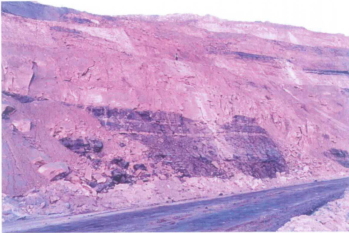
Photograph showing slide, crushing of benches in OB & Coal.
