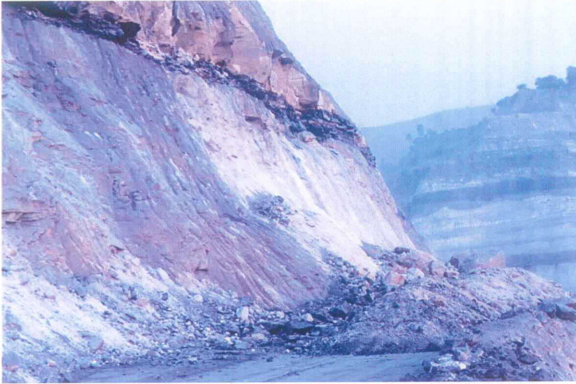
Photograph showing slide, crushing of benches in OB.
